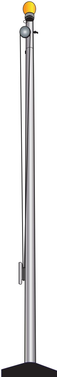
What if you could clip the flag to hooks on a rope and fit the rope into wheels at the top and bottom of the pole? Then you could just pull down on one side of the rope, causing the other side of the rope to raise the flag. Problem solved!
